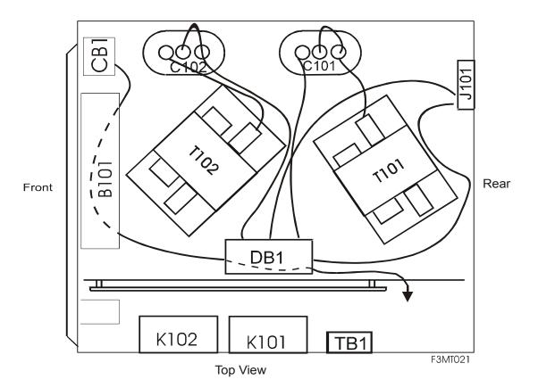
Figure 47. P300 MT HV Wiring
